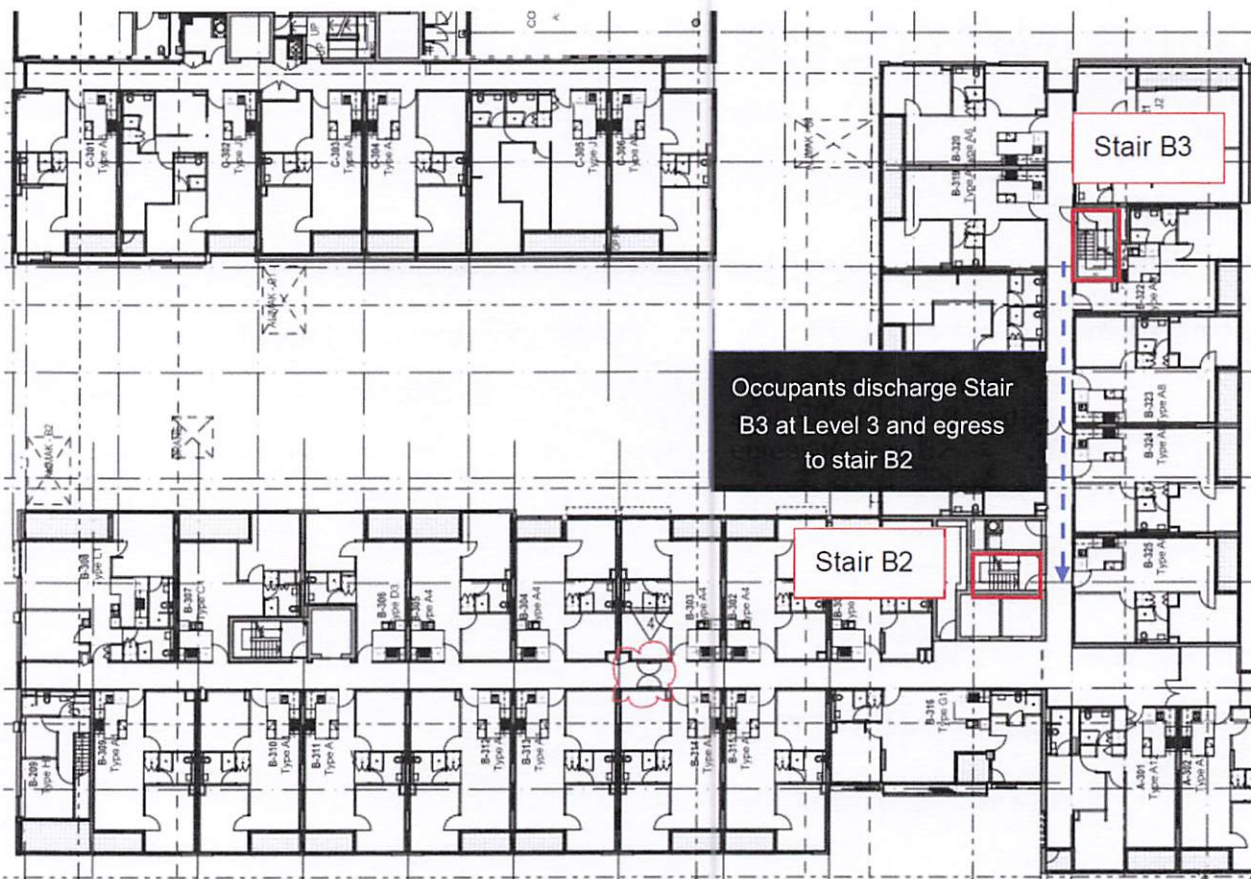
Figure 1: Internal discharge of stair B3 at level 3
